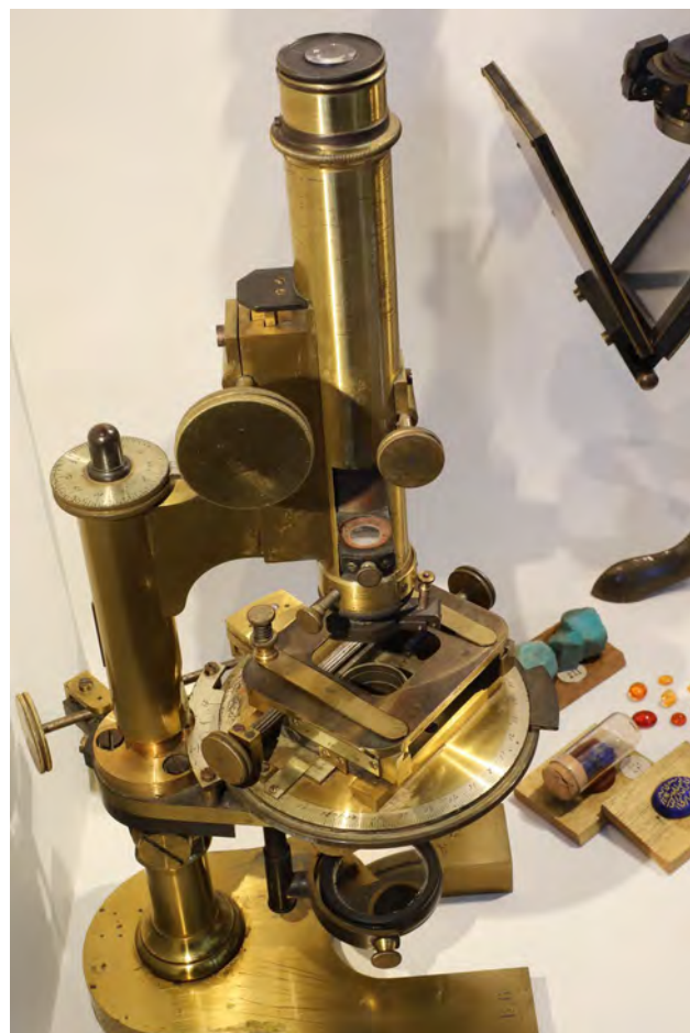
One of Emile Bertrand's microscopes, equipped with a "Bertrand lens". Bibliothèque Mines Paris – PSL.
